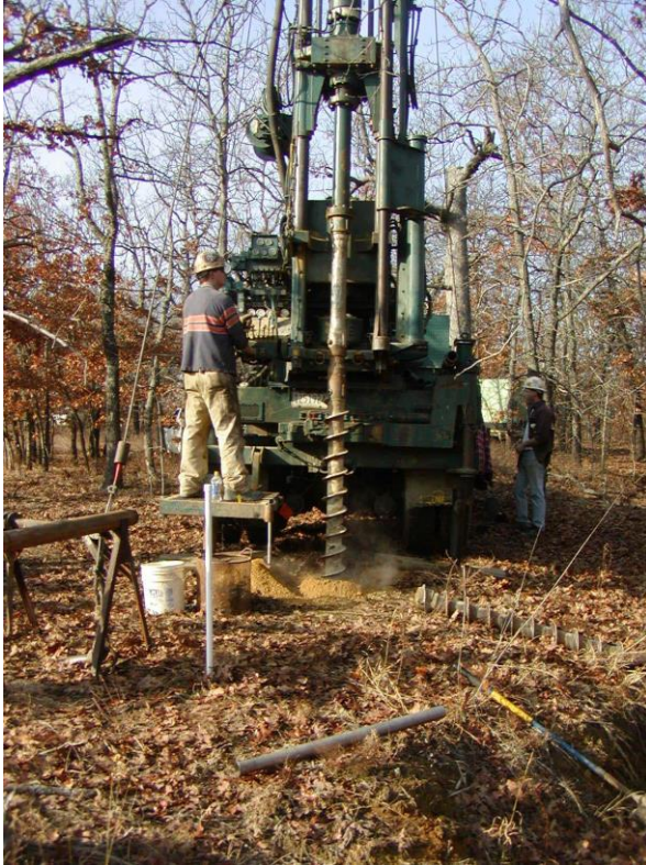
Photo 1: Typical Auger Drill of the scale required for this prospecting operation (Source: USGS, 2012)
