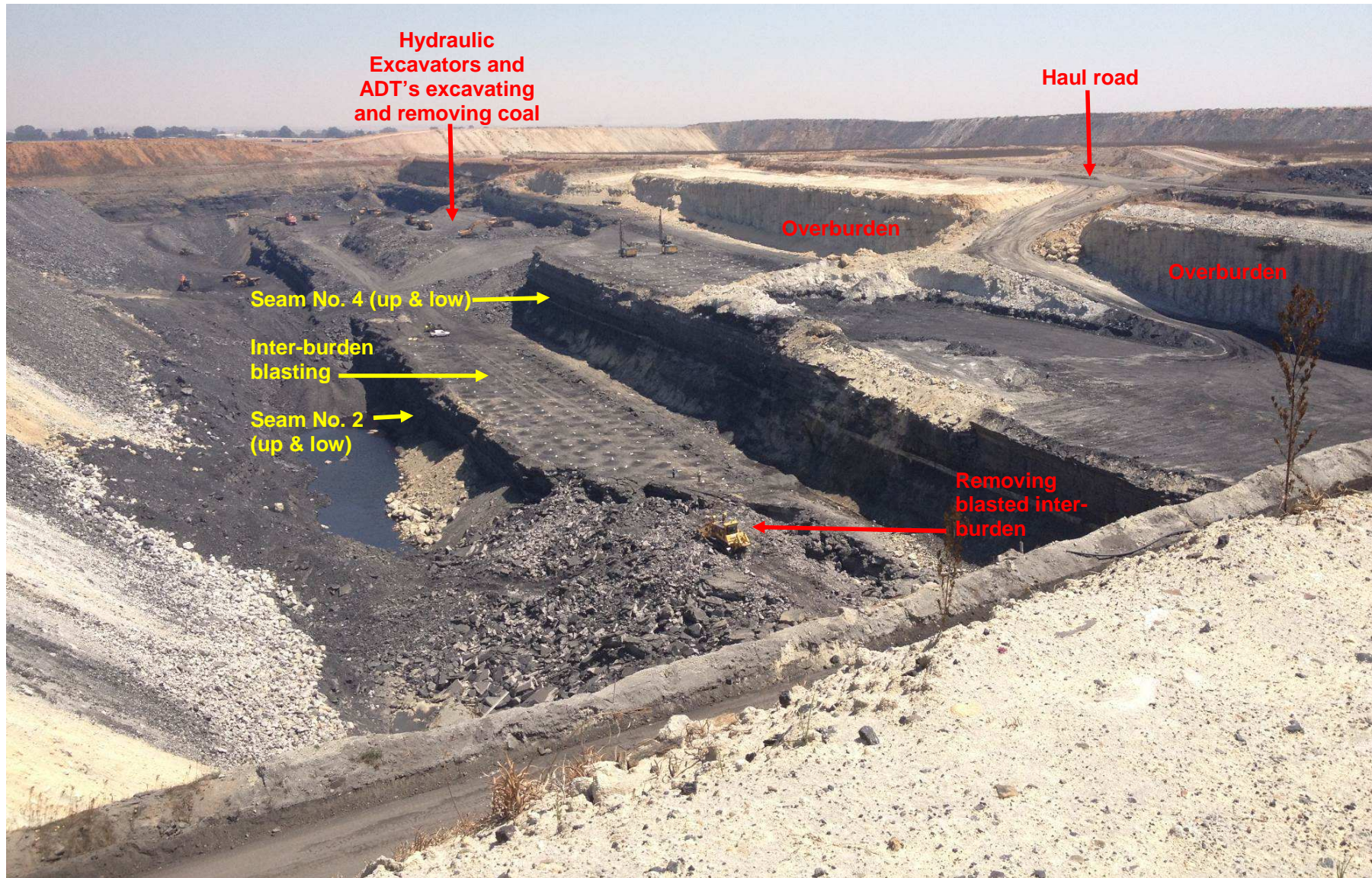
Figure 4: Opencast Coal Mining Process (Vlakfontein Central Block)
