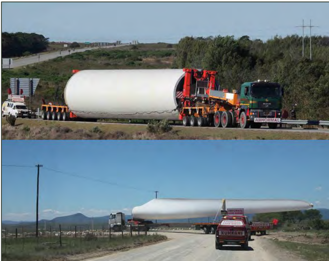
Figure 3: Abnormal freight (tower section in low-load configuration (top), and blade (bottom))
