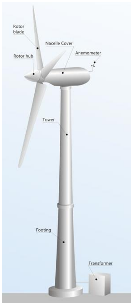
Plate 2-1: Typical example of wind turbine structure and components.
