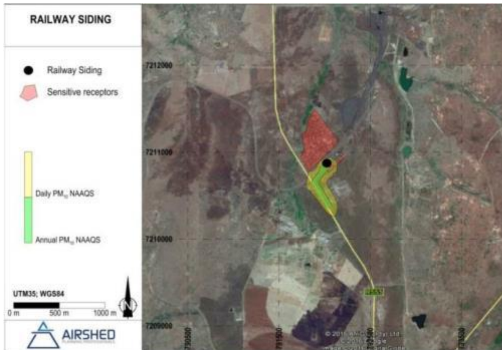
Figure 88: Area of exceedance of PM10 NAAQS due to mitigated railway siding operations
