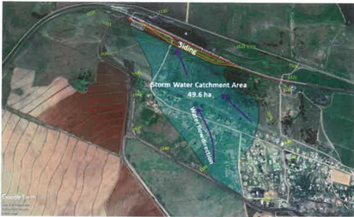
Figure 8.3-10: Storm water catchment area
