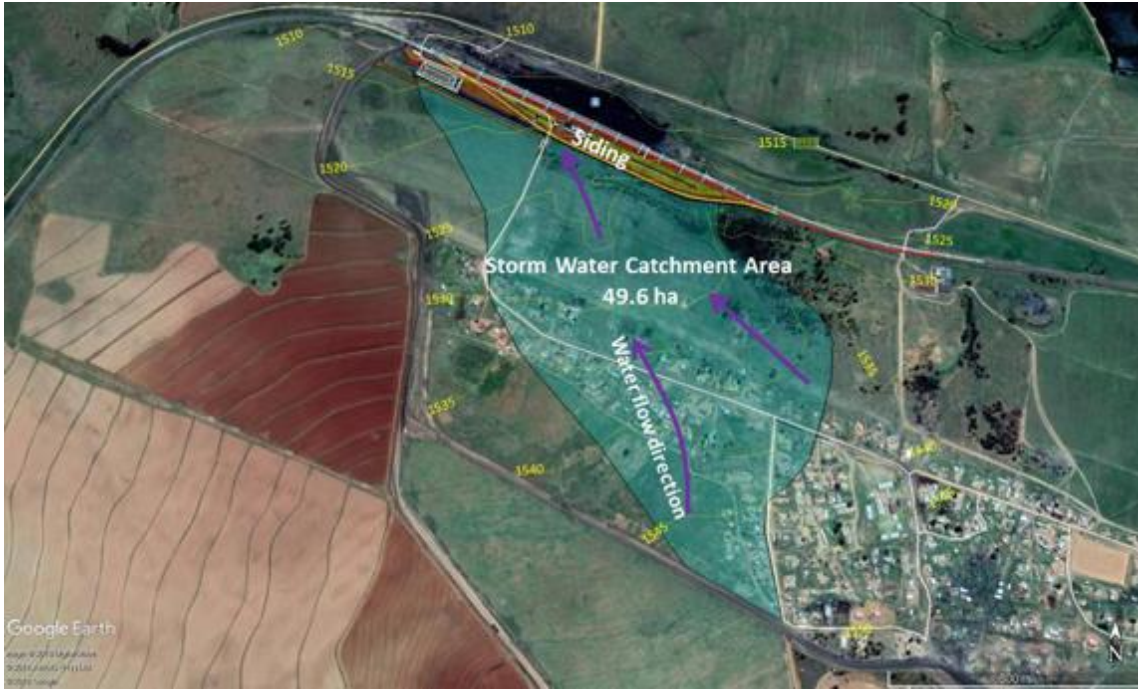
Figure 6.1-17: Storm water catchment area
