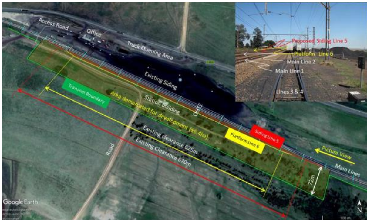
Figure 6.1-5 Proposed site for the future increase in scope of the existing railway siding.
