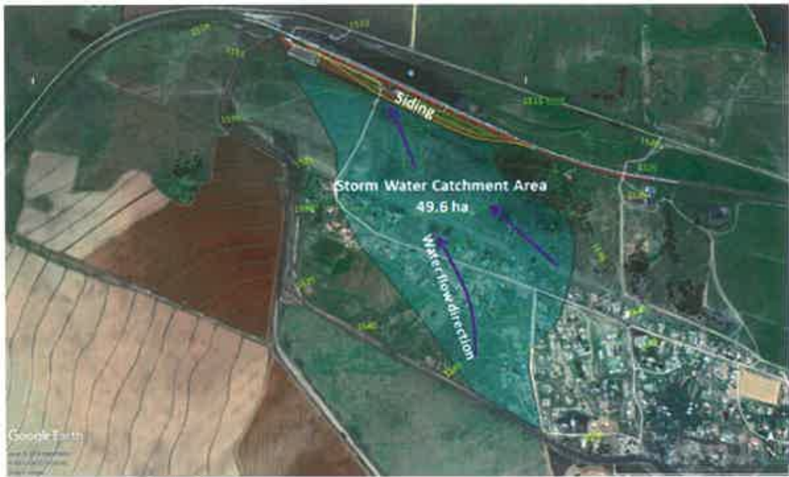
Figure 6.1-17: Storm water catchment area
