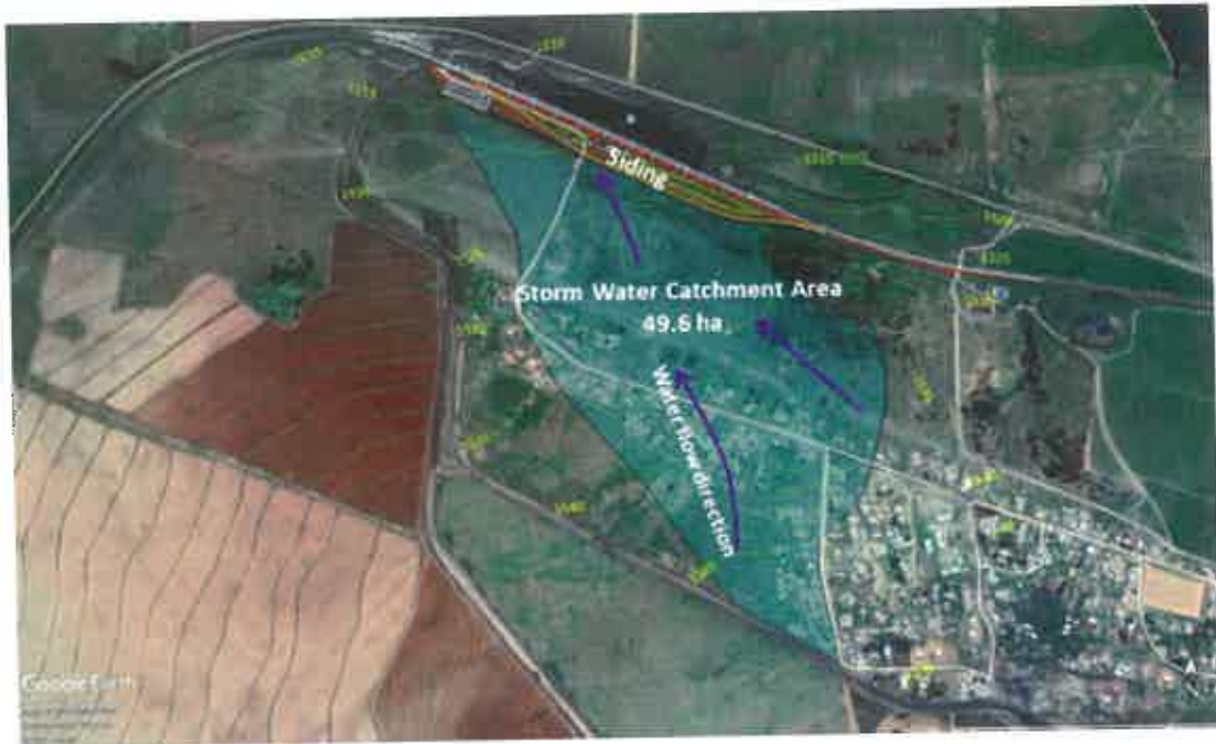
Figure 6.1-17: Storm water catchment area
