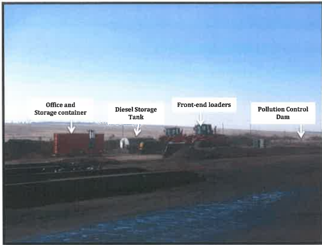
Photograph 2.3-3: The infrastructure and machinery on the current operations within the Northern side. The Container is an office and storage, the diesel storage tank and heavy machinery - front end loaders parked behind the soil berm. The Pollution Control Dam (PCD) is also visible fenced in at far right hand side.
