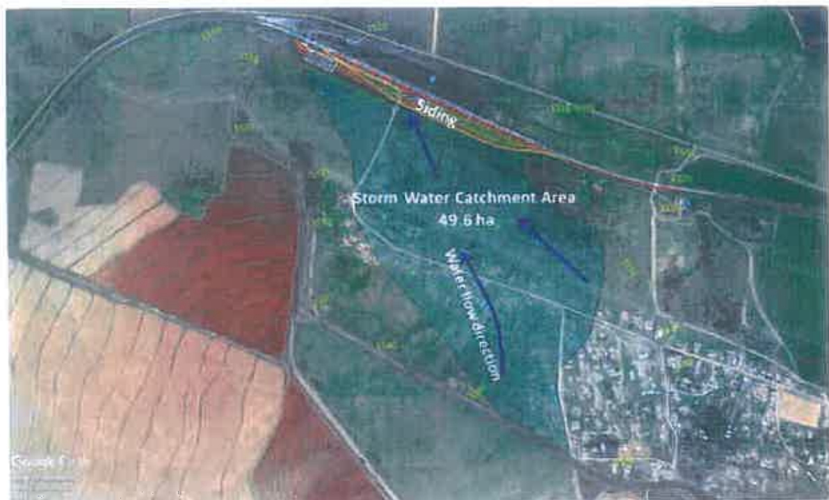
Figure 14: Storm water catchment area
