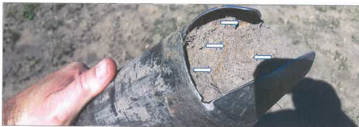
Figure 7: Orange rhizospheres and mottles (arrows) observable in the transition between the orthic and albic horizon of an augered soil sample from the temporary zone of the hillslope seepage wetland
