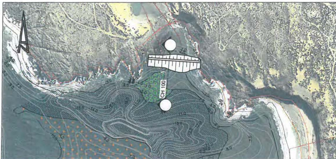
Figure 5.1: Northern channel closure berm concept
