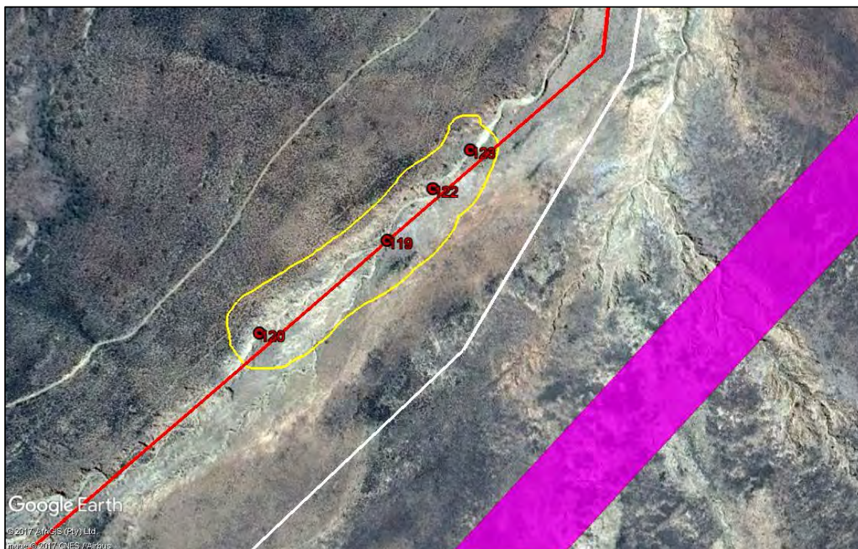
Fig. 39. Detail of the south-western sectors of the 132 kV powerline routes shown in the previous figure. Alternative 1 (red line) passes through the proposed 50 m-radius protective buffer (yellow shape) surrounding several important fossil vertebrate burrow sites in the Katberg Formation that are exposed in a deeply-incised stream bed (Locs. 119-123). Alternative 2 route option – white. Preferred route option – purple.
