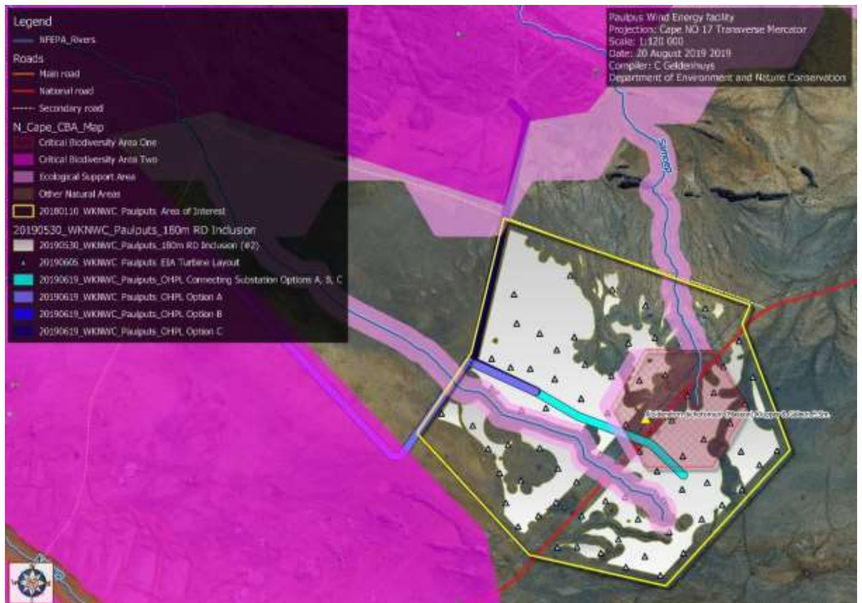
Figure 1 Layout of the proposed Paulputs WEF in the context of environmental sensitivities: CBA areas and buffered habitats / sensitivities (the grey-white polygons indicate assessed areas suitable for turbines).
