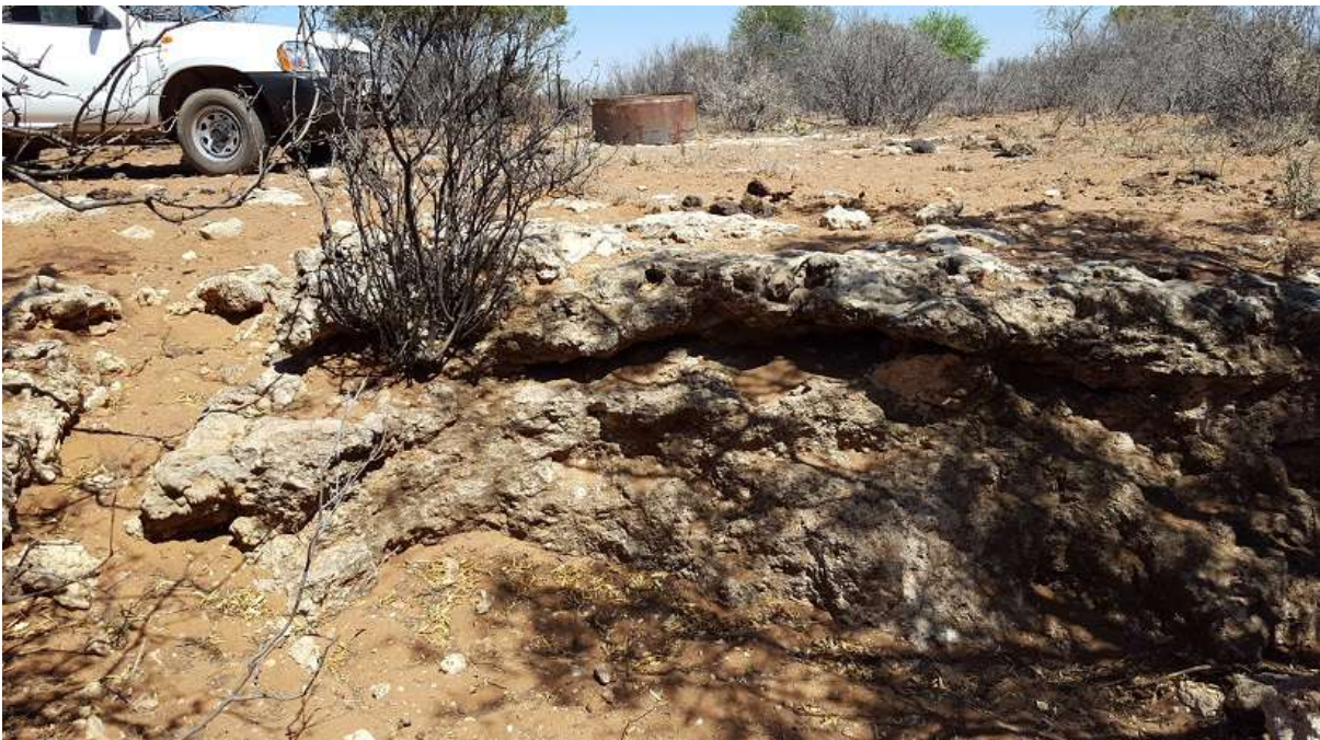
Figure 5: Photograph showing an exposure of the hardpan carbonate layer that is dominant across the site.
