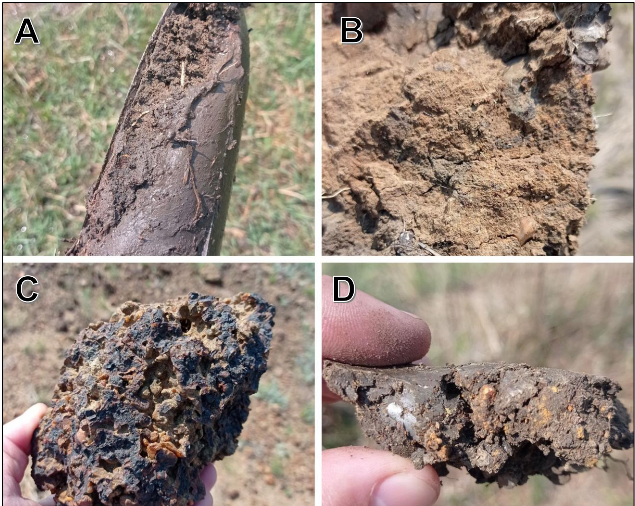
Figure 8-32: The soils within the project area. A) Katspruit soil, B) Mottled Westleigh soil, C) Hard Plinthite layer, D) Wet Glenrosa soil. (October 2022).
