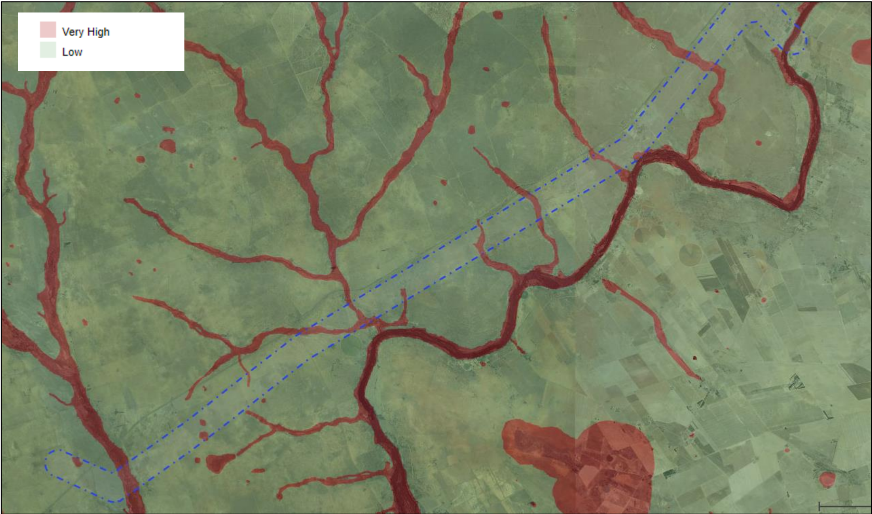
Figure 5-1: DFFE screening tool results for the aquatic biodiversity sensitivity theme for the project extent.
