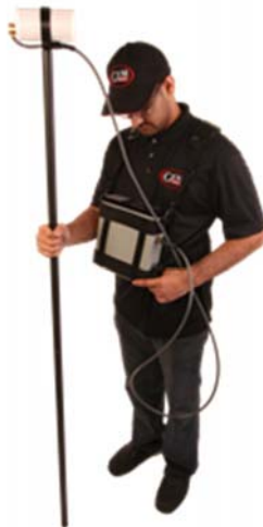
Figure 4: GSM-19T Proton Precession system in action.
