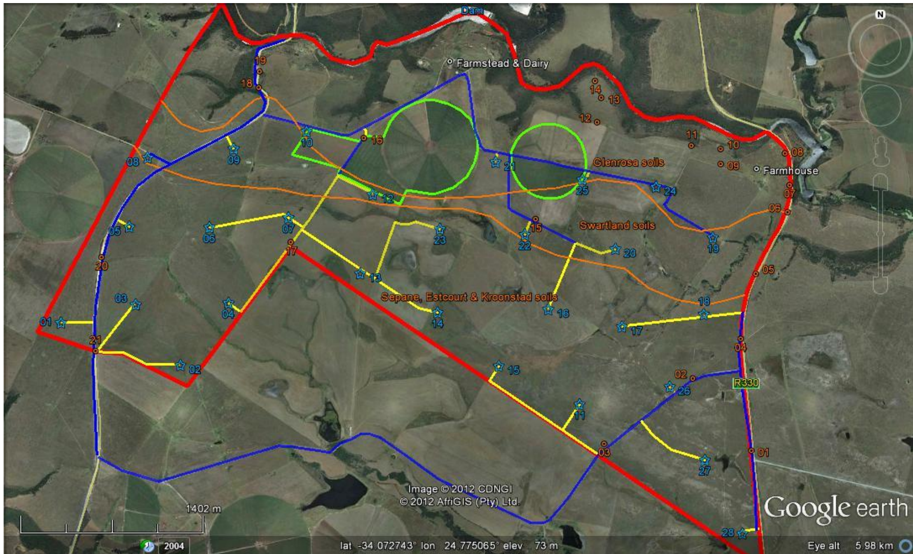
Figure 14.2a: Site Plan of Banna Ba Pifhu Wind Farm for alternative 1 (50 MW, 27 turbines). Turbine positions and numbers in light blue, existing roads in blue, new roads in yellow, irrigation lands outlined in green, soil lines and sample numbers in light brown. Details of all soil sample points are provided in Appendix 14.1.
