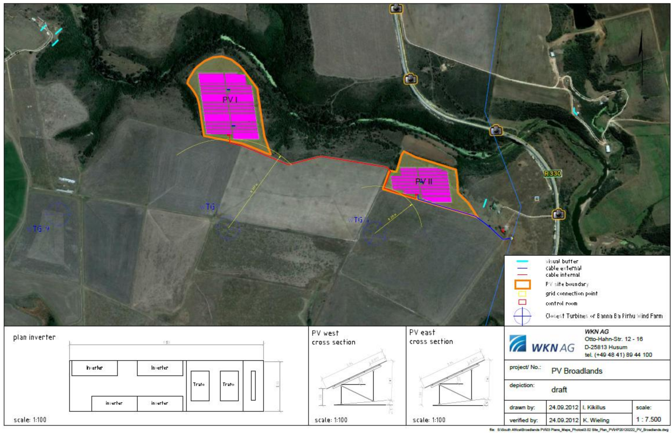
Figure 2.4 : Layout of the proposed PV facilities and the distance of the closest wind turbines that form part of the Banna Ba Pifhu wind energy project.
