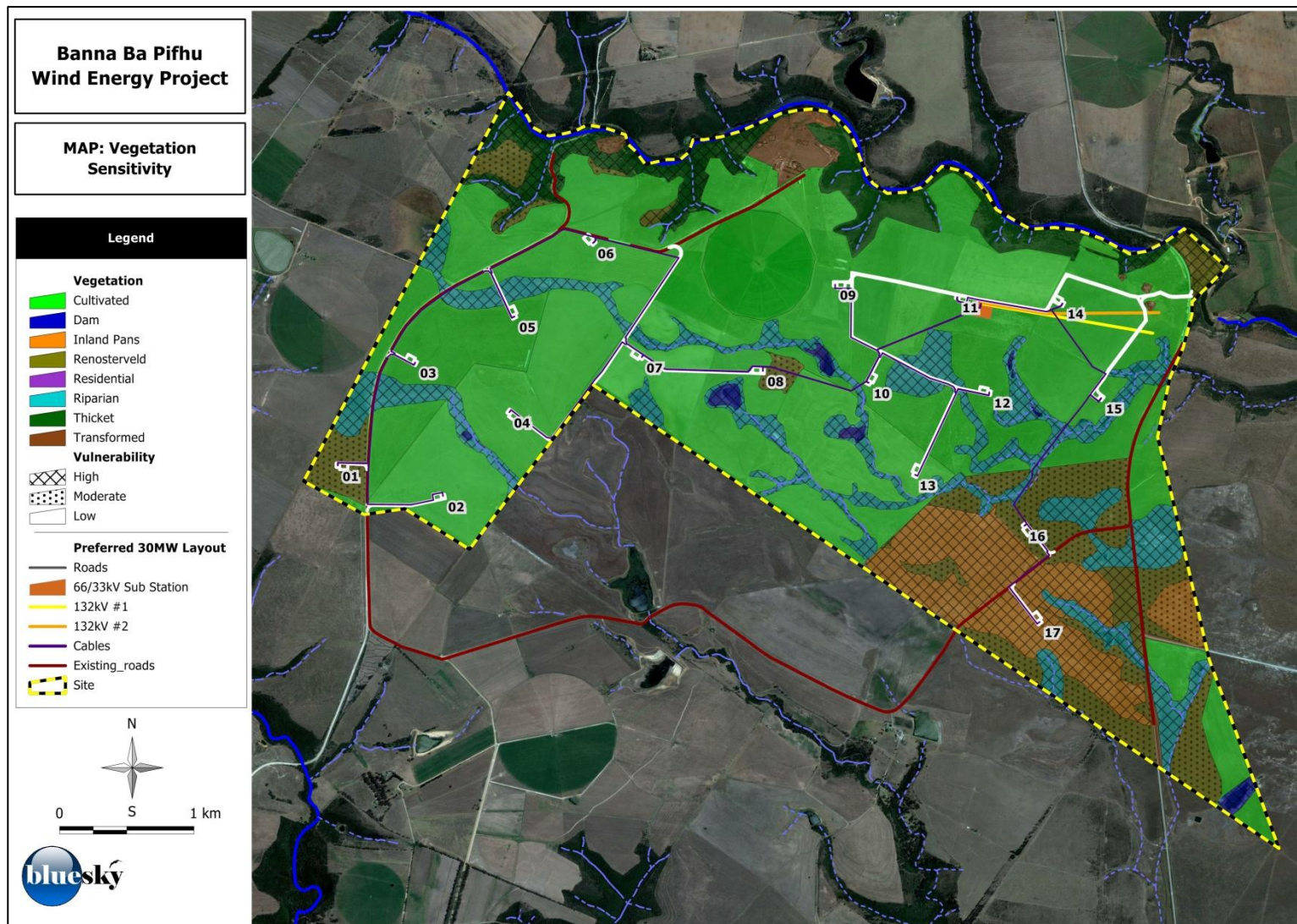
Figure 5-40: Mapped Vegetation communities with preferred alternative 30.6 MW layout overlain for maximum number of sites (17 turbines).
