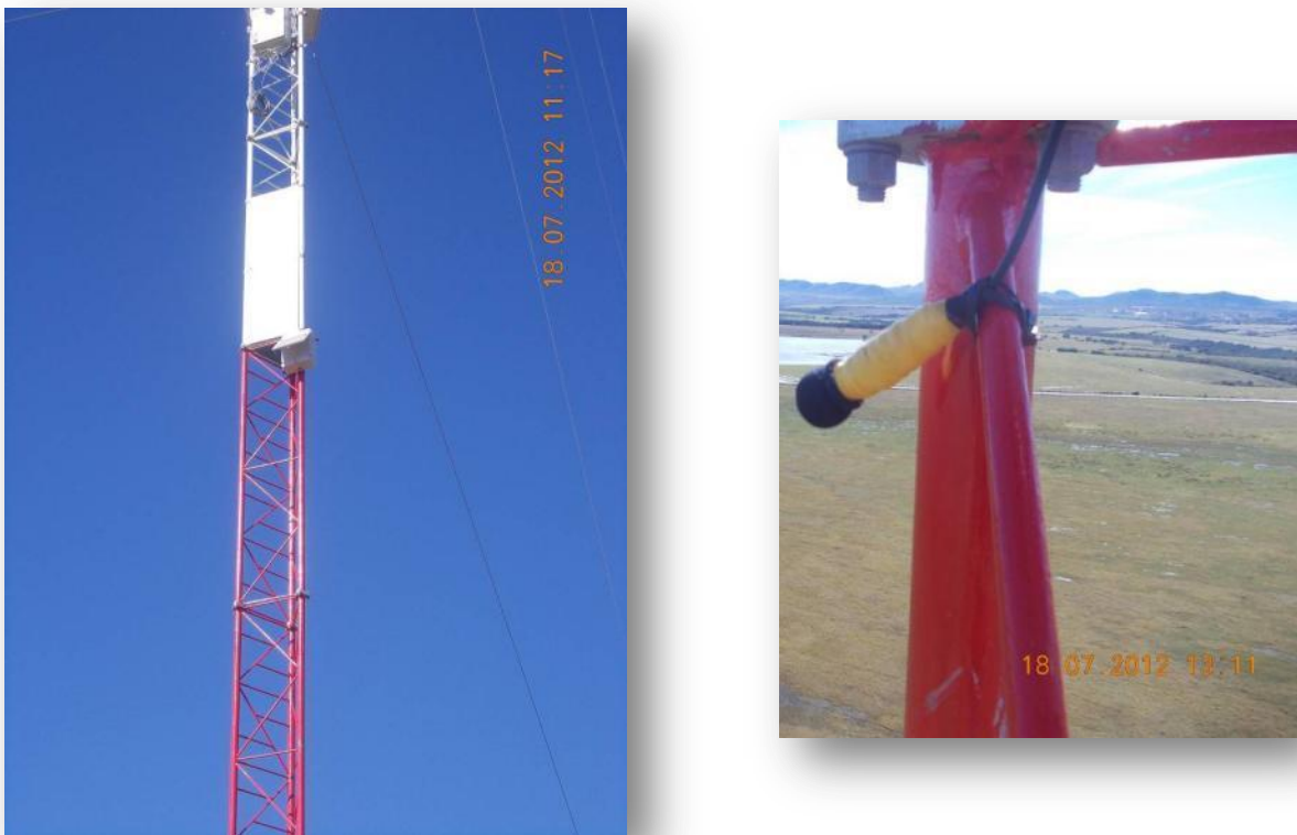
Figure 7-4: Met Masts with the 192kHz SM2BAT Detector and Microphone at 10 m and 60 m respectively
