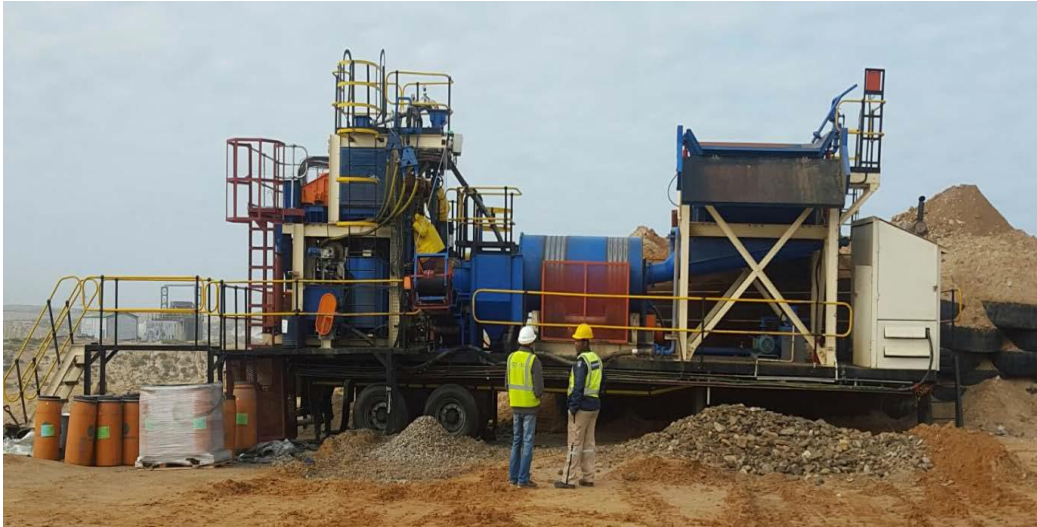
Photo d - 4: New WCR 10tph mobile DMS Prospecting Plant in transit (top) and in operation (bottom)
