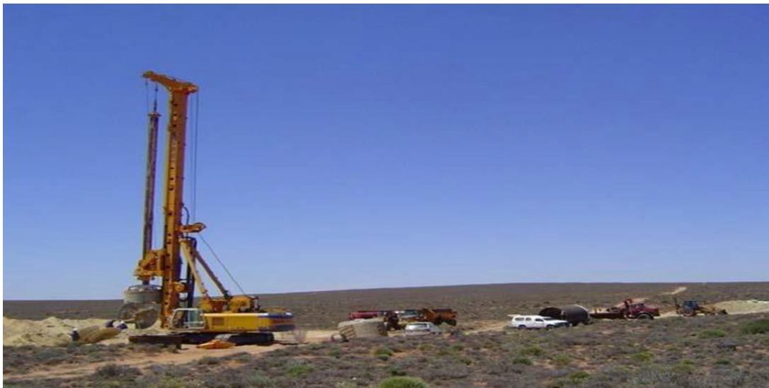
Photo d - 2: Bauer BG36 auger drilling system employed from the late 1990's
