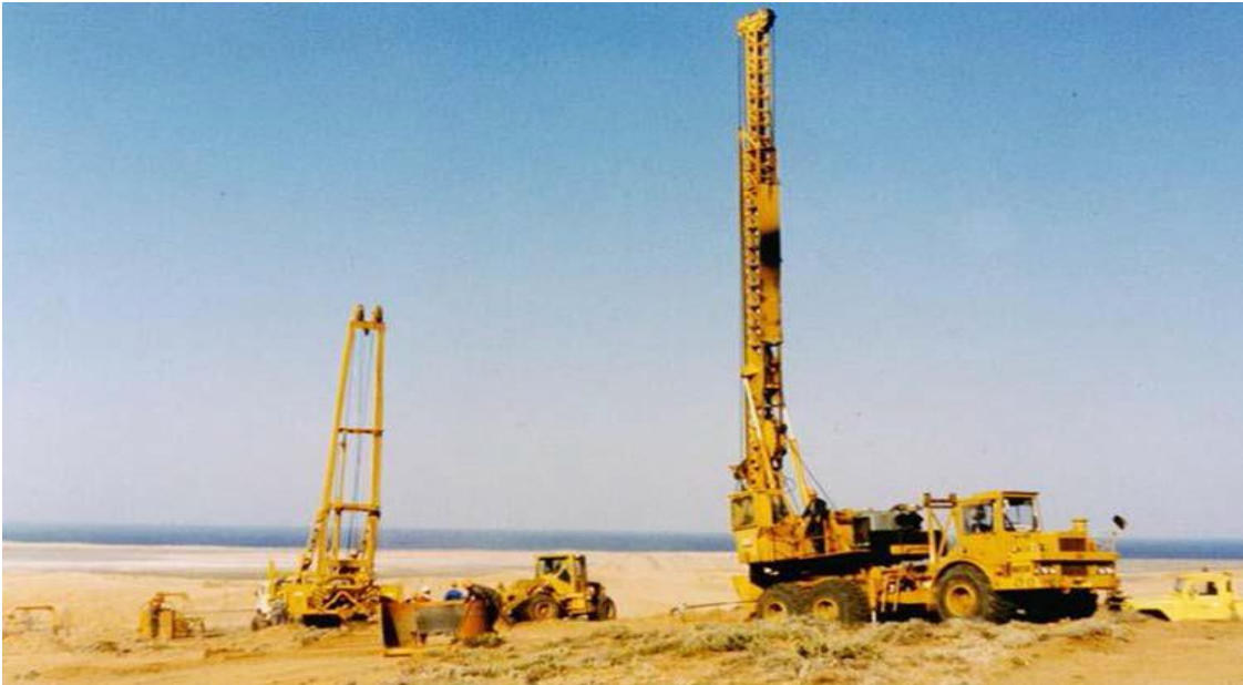
Photo d - 1: Soilmec auger drilling system employed until the mid-1990's
