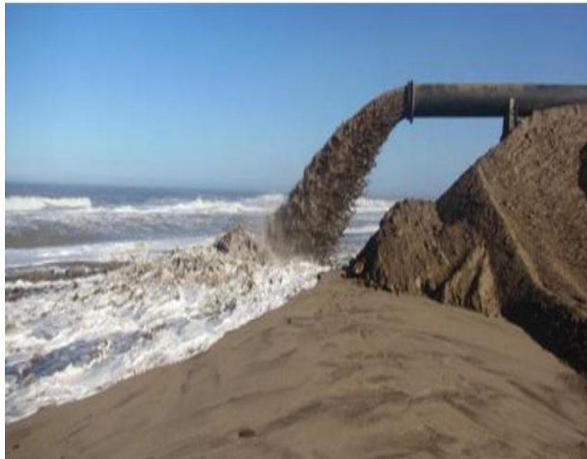
Illustration 2: Diagram illustrating the hydraulic mining method (top) and discharge of slurry to sea for beach accretion and seawall mining (middle and bottom).
