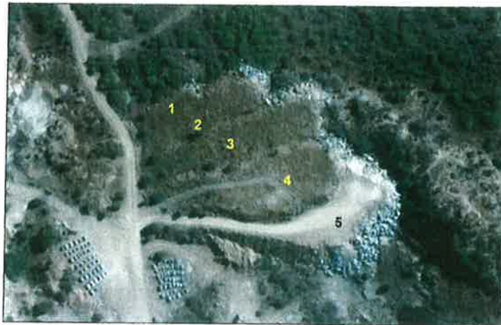
Figure 10 e is an aerial view of five established terraces at Wonderkop 1. Terrace 5 represents the active section of the waste rock dump (MRD 1/Mine residue deposit 1).
