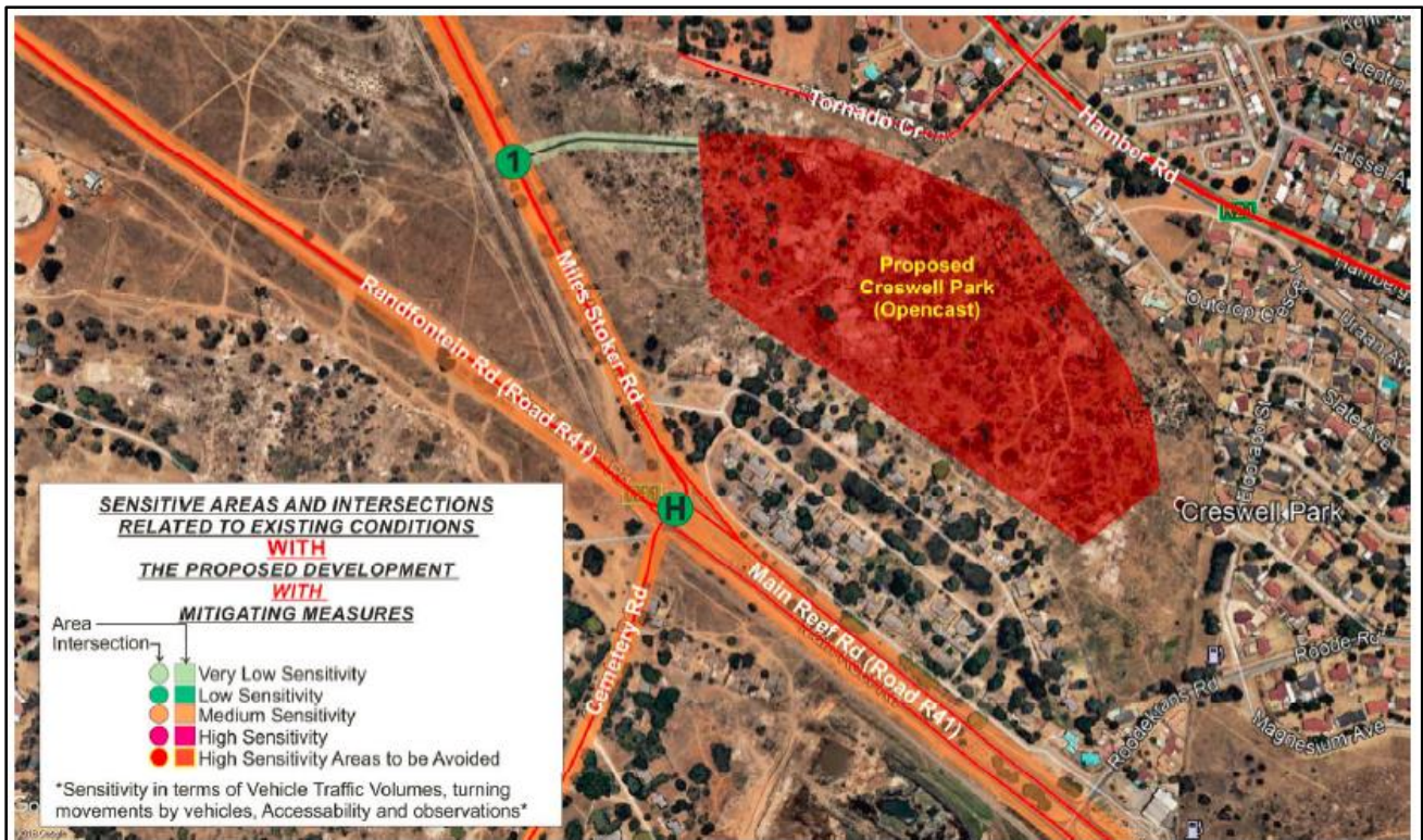
Figure 44: Presentation of existing sensitive road sections and intersections with background mitigating measures with proposed mining development
