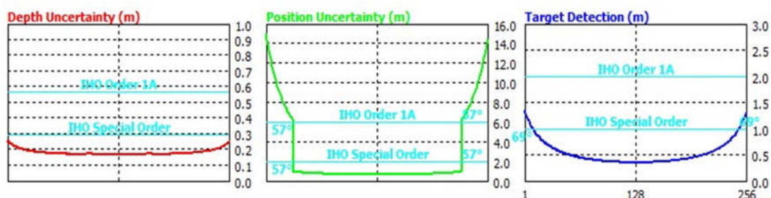
Figure 14 - report generated using the TPU utility showing Odin fitted with the Norbit iWBMS and RTK positioning system achieves the minimum IHO standards.
