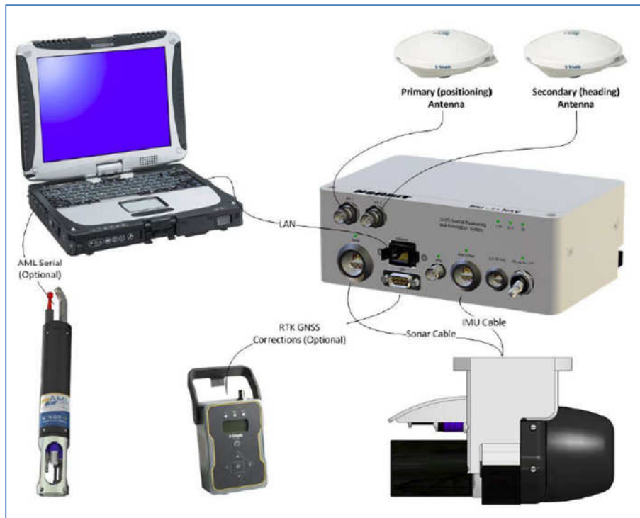
Figure 11 – Norbit iWBMS multibeam equipment flow diagram
