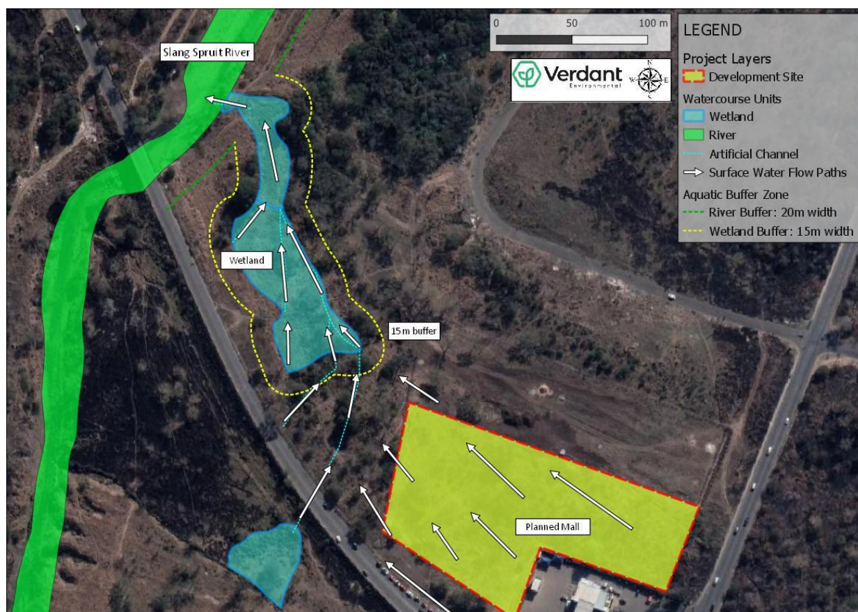
Figure A. Map showing location and extent of the Slang Spruit River and Seep Wetland downstream to the west of the Mageza Mall development site, with recommended 15m wetland buffer zone and 20m river buffer zone also indicated.
