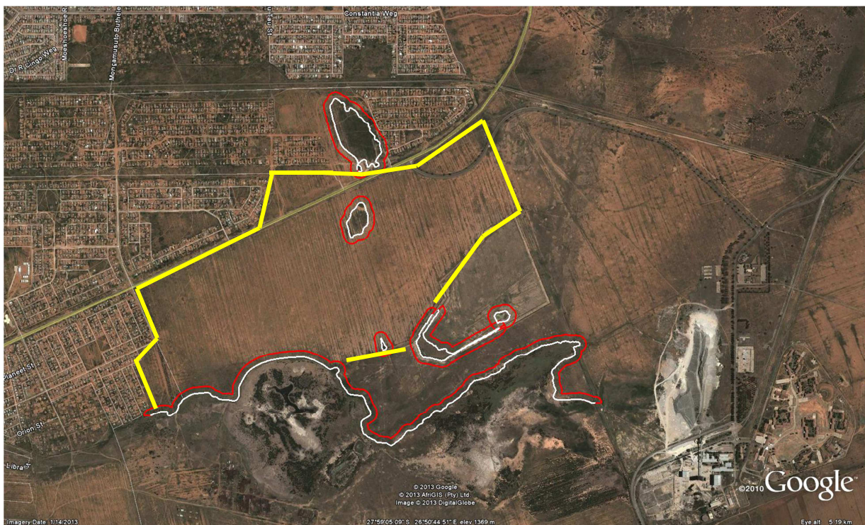
Figure 4: A map showing the delineated wetland areas (white line) in the study area. The red lines indicate the wetland buffer zone. Yellow lines indicate area of proposed development.
