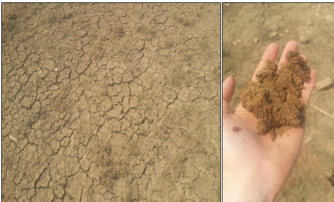
Figure 36: Cracking Clays (left) and Soil Sample showing Orange Mottling (right) in the Soil Matrix
