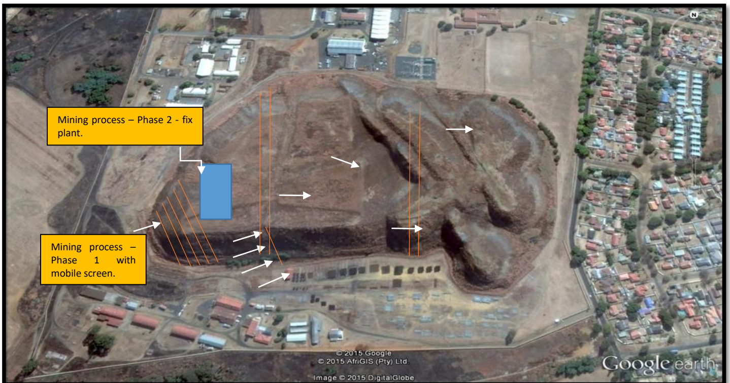
Figure 1: Picture showing the location of the reclamation plant for the two proposed reclamation phases
