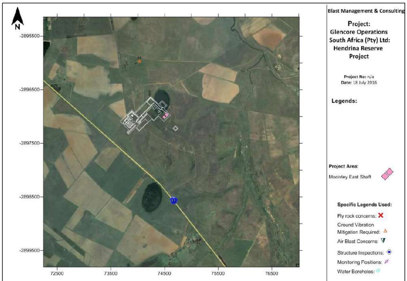
Figure 34: Structures identified where ground vibration mitigation will be required at Moovley East (Shaft No. 3).
