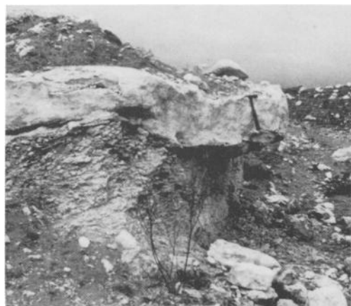
FIG. 6. Hardpan calcrete overlying nodular calcrete (Netterberg 1980).
