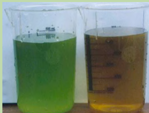
Vetiver grass will remove phosphate and nitrate from polluted water. The beaker on the left is before treatment; on the right 4 days later 90% P and 94% N removed
