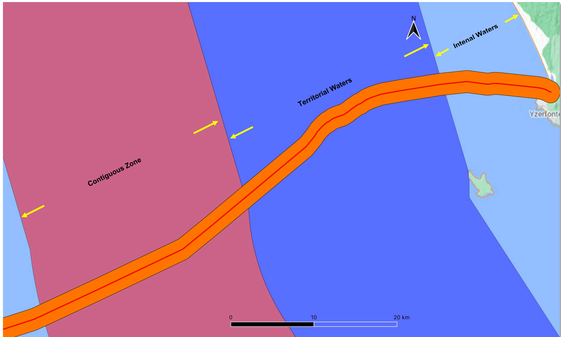
Figure 5: Maritime archaeological assessment study area for this report between the outer limit of the contiguous zone (24 NM from the baseline) to the mean high-water mark at the landfall at Yzerfontein. The study area comprises a 1 km buffer (orange) on either side of the proposed cable route (red line). (Source: Google Earth).
