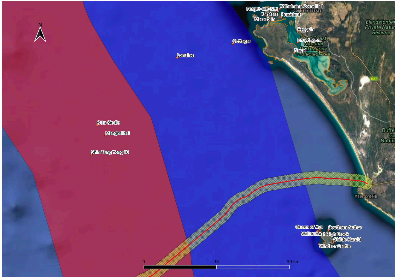
Figure 13: Proposed alignment of the 2AFRICA (West) cable system showing the relative positions of the concentrations of wrecks around Saldanha Bay (top) and Dassen Island (bottom) (Source: Google Earth).
