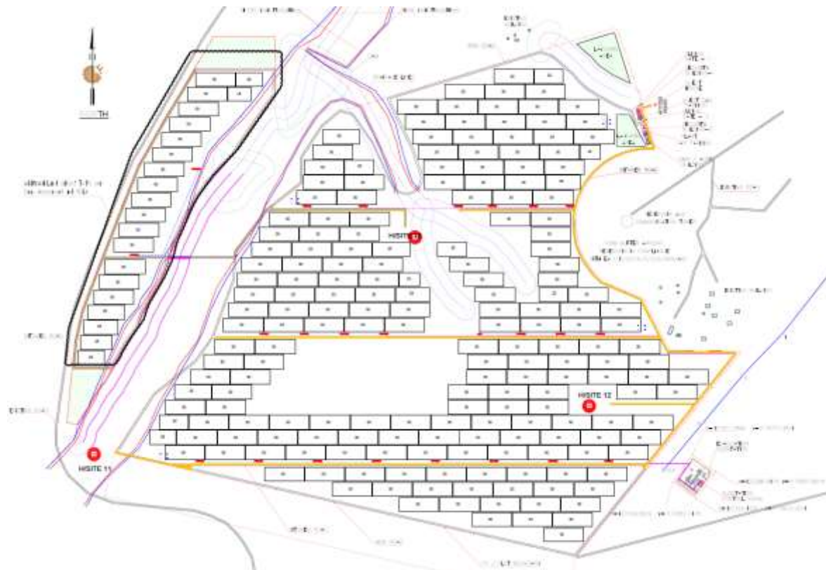
Figure 8: General Site Plan utilising only the area west of the drainage and line (Alternative 2)
