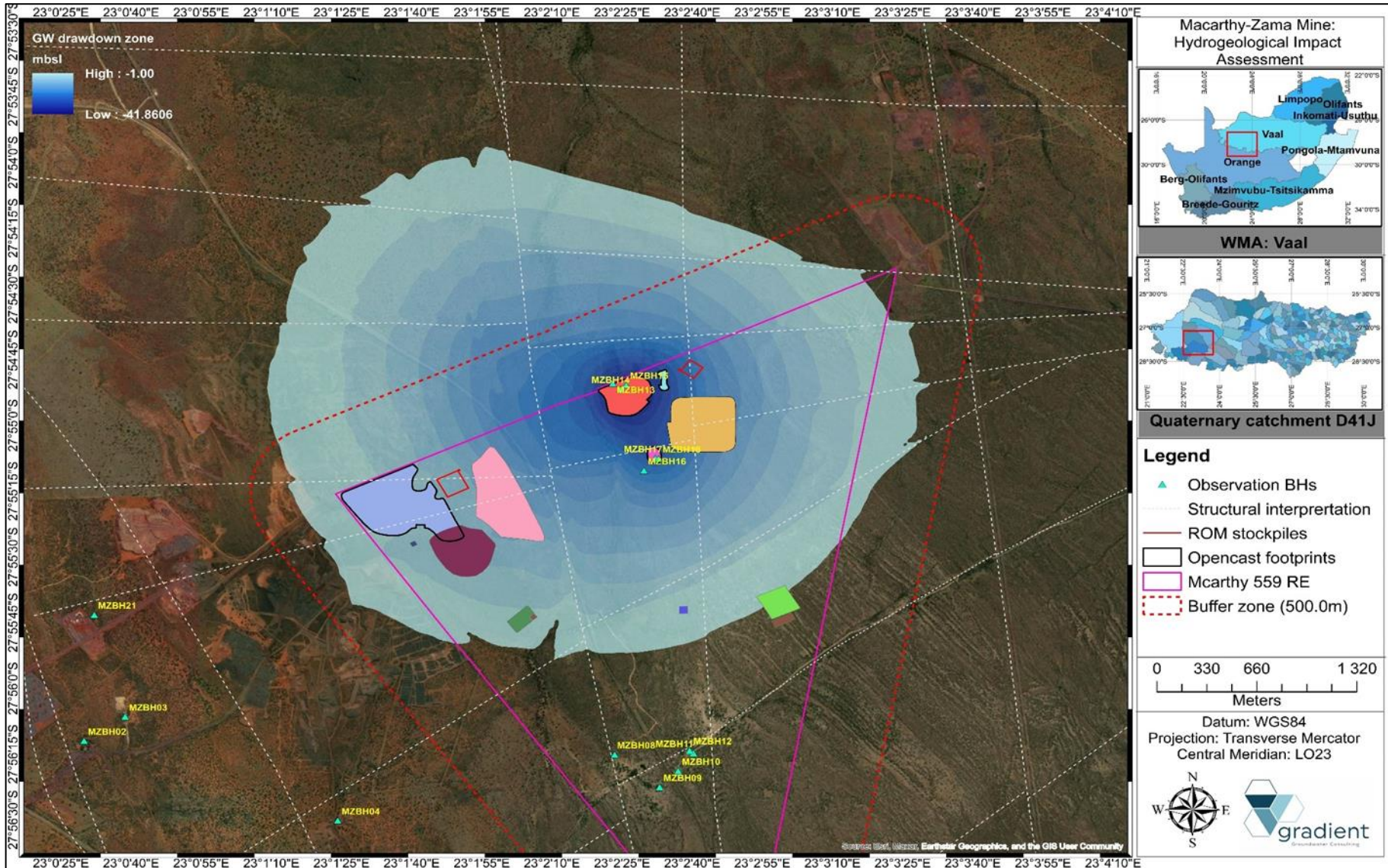
Figure 11-7: Water level drawdown and groundwater capture zone of the host aquifer formed by opencast dewatering activities for the LOM operational phase.
