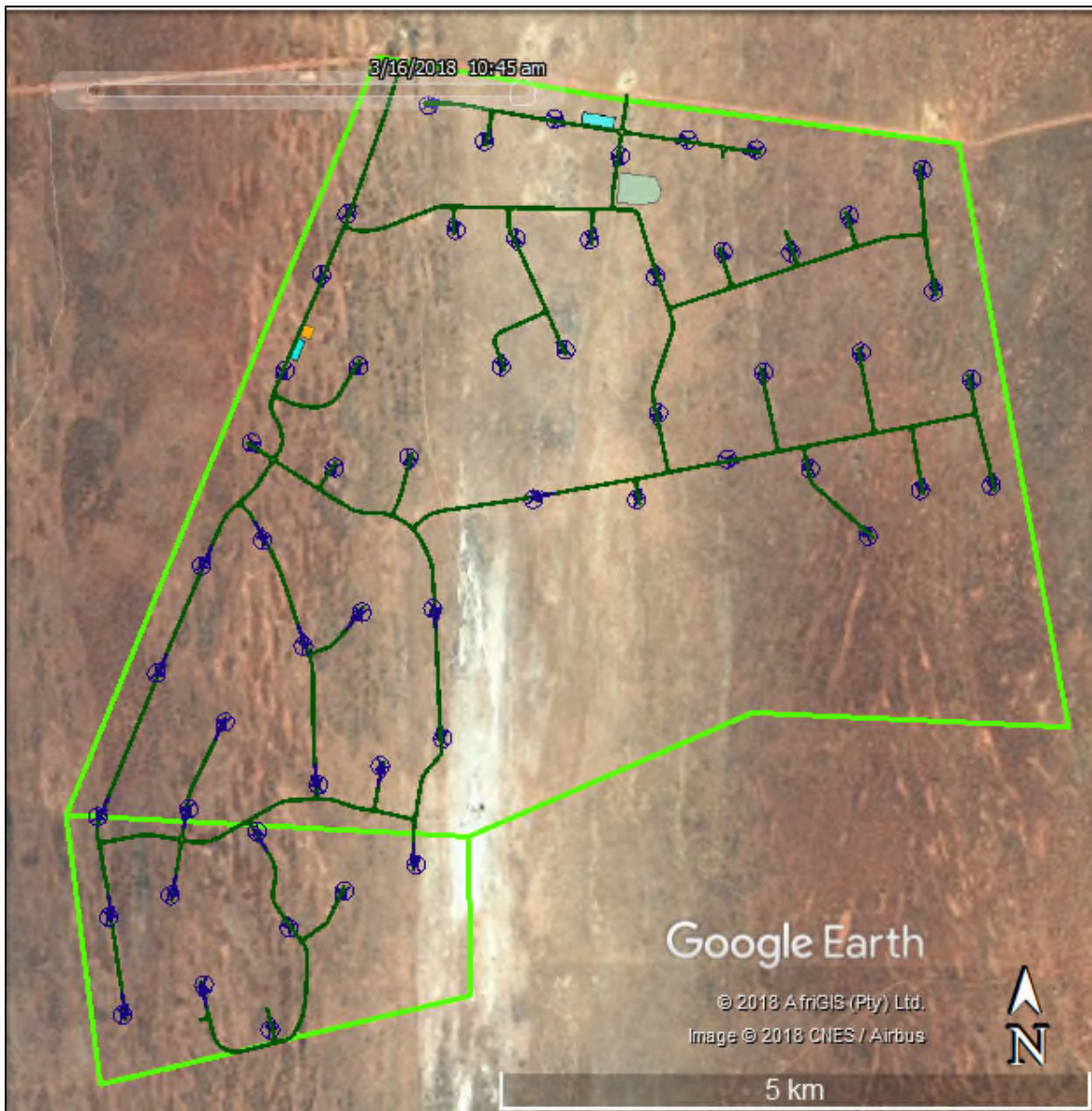
Figure 2: Aerial view of the study area showing the proposed facility layout (turbines marked in blue, roads in green, substation in orange, laydown area in light green and two offices in turquoise).
