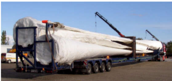
Figure 3-2: Example: 3 x 45m Blades on extendible trailers 2
