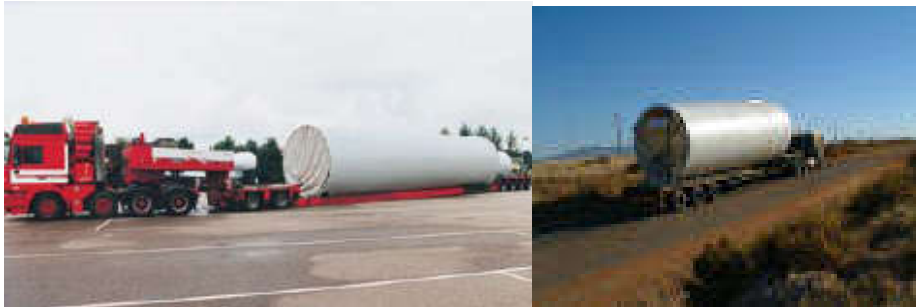
Figure 3-4: Transporting the Tower Sections (Source: Author's photograph)
