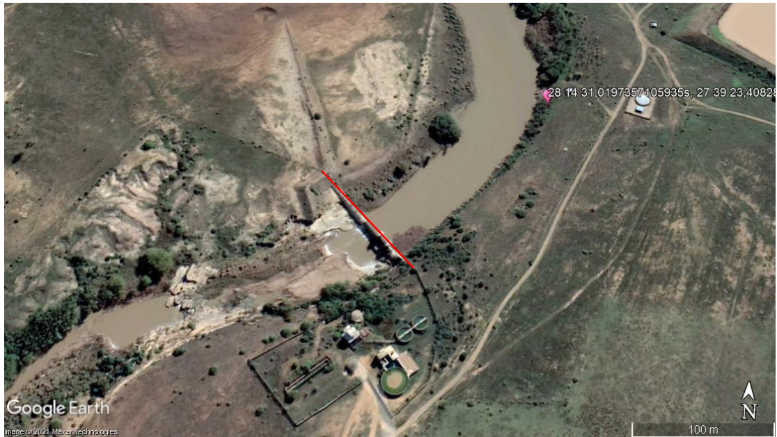
Figure 9: Aerial view of the abstraction works which clearly indicates the effect the weir (red) has had on the river and its banks when looking upstream and downstream of this weir (Google Earth 2021).
