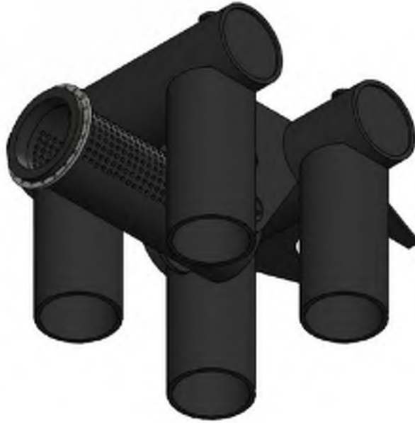
Figure 17 – Isometric View of HDPE Floating device for Water Abstraction – with Stub Flange for Connection to PE 100 DN 710mm HDPE Pipe
