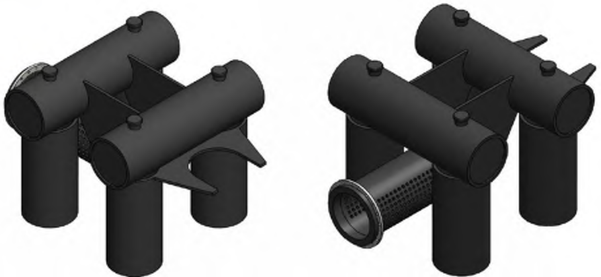
Figure 16 – Isometric View of HDPE Floating device for Water Abstraction – with Stub Flange for Connection to PE 100 DN 710mm HDPE Pipe
