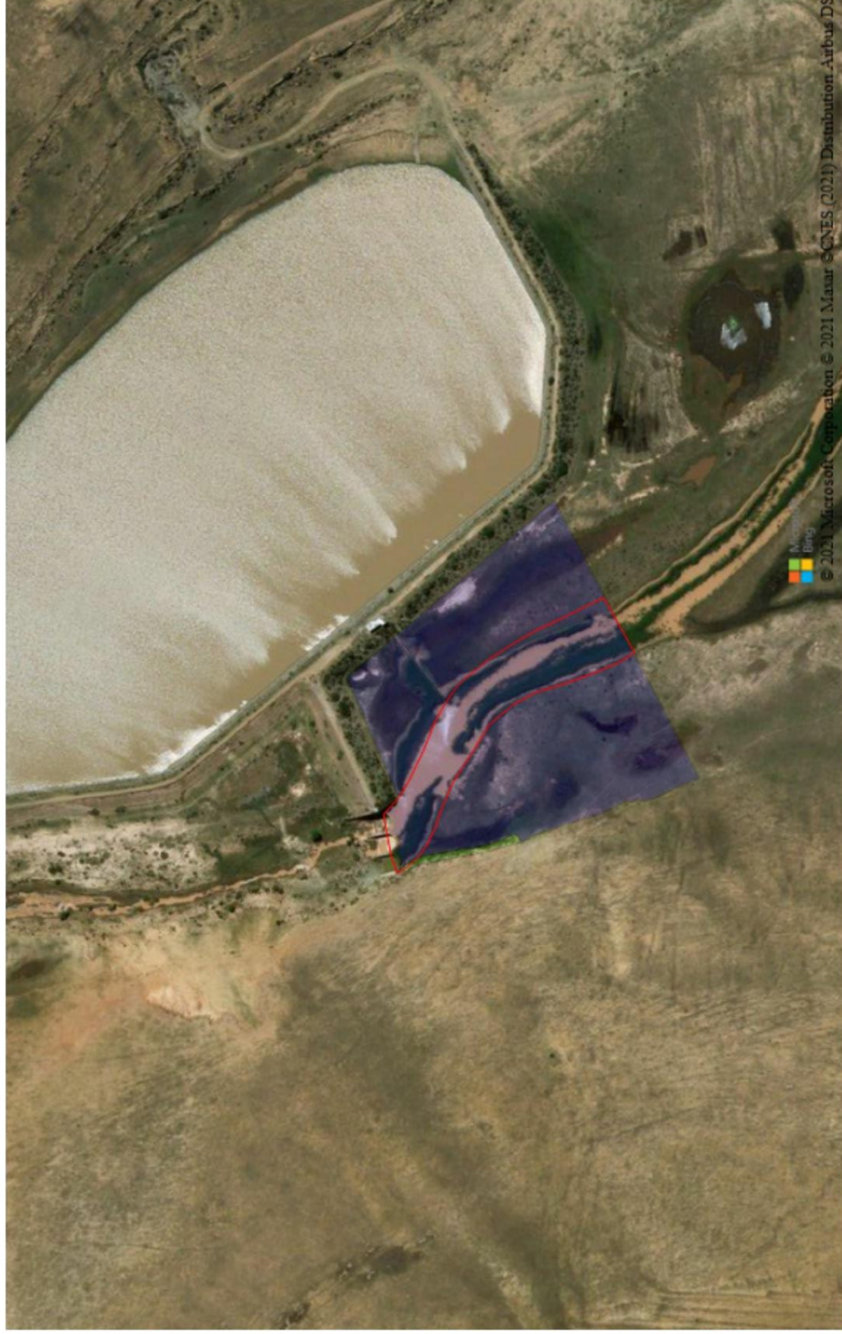
Map 1: Wetland delineation map for the proposed dredging operations within the Sandspruit. The De Put off-channel dam and associated weir is clearly visible. The course of the Sandspruit and the footprint of the proposed dredging operations are also indicated. Note the extensive wetland areas associated with the river. The wetland areas around the proposed dredging site has been delineated and cover the entire floodplain, up to the toe of the damwall. Note also the section of riparian zone along the western banks of the river which is indicative of the border of the floodplain and surrounding terrestrial areas.
