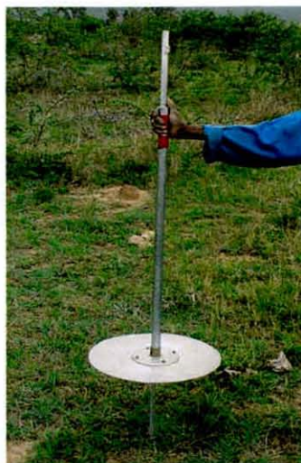
Figure 2: The disc meter, developed by Bransby & Tainton (1977) to determine the standing grass phytomass. Grazing volume is expressed in kg/ha or tons/ha.
