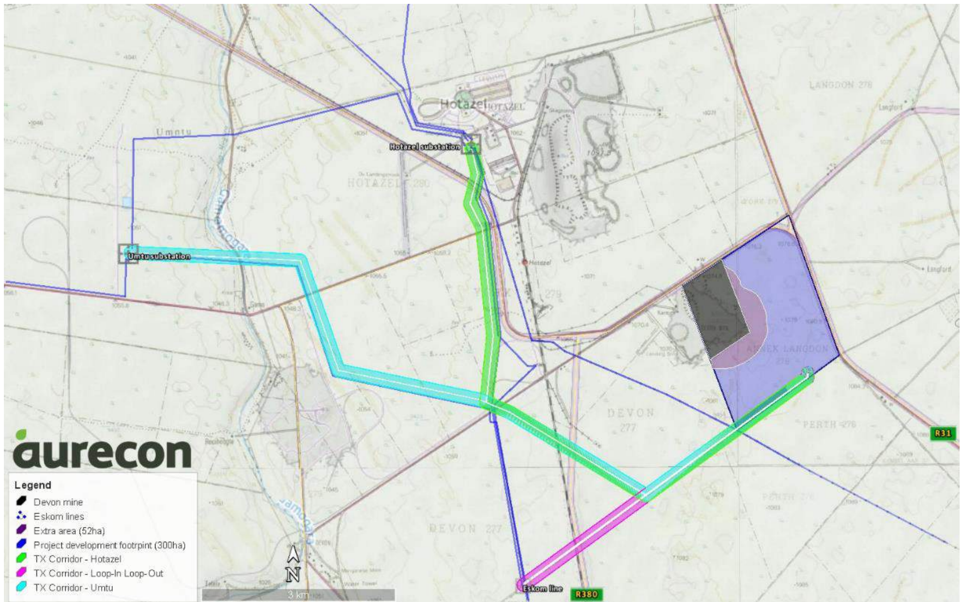
Figure 26. Transmission line alternatives to evacuate power from Hotazel Solar Park (Map supplied by Aurecon).
