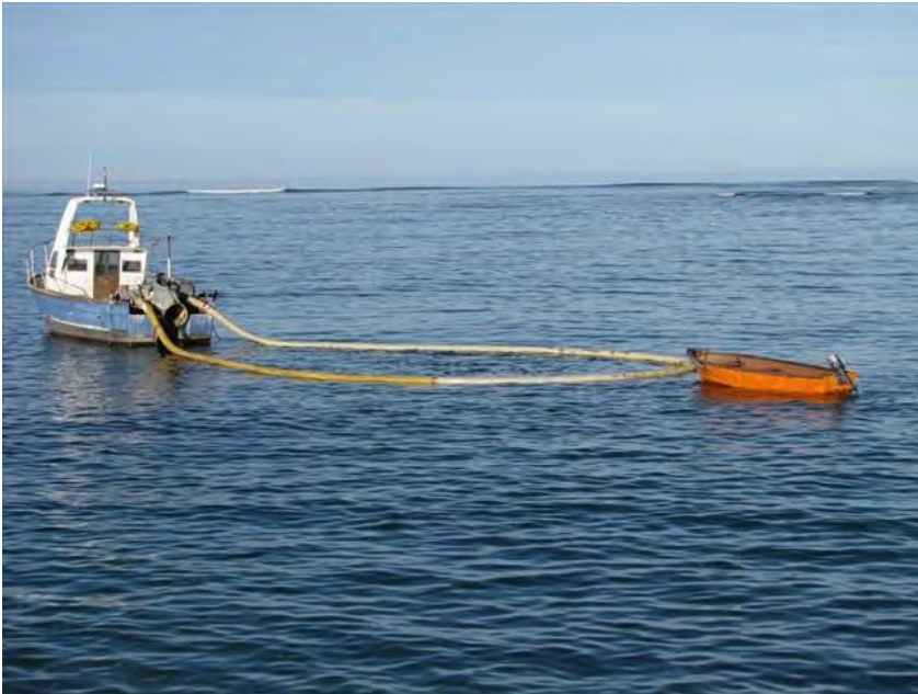
Figure 2-5: Ski boat with fitted suction hoses
