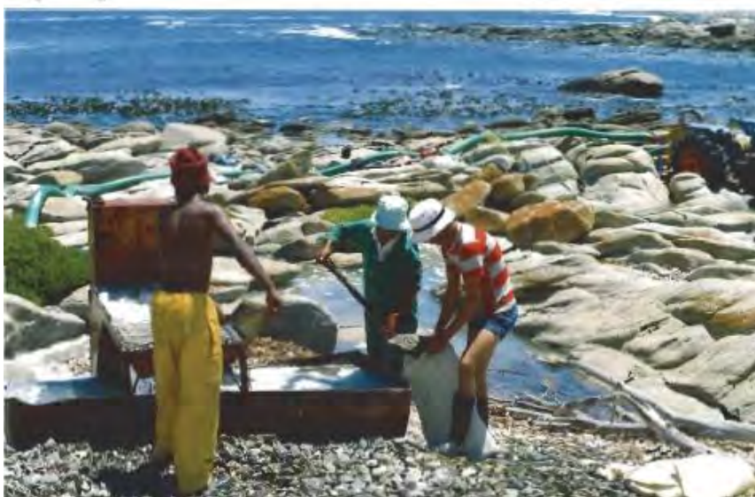
Figure 2-6: The other end of the suction apparatus illustrated in Figure 2-4 will be mounted on a tractor (which supplies the power) that is located nearby, together with a sieving operation. The sack in the foreground contains diamond-bearing material that has been screened to eliminate the coarse gravel. This "sieved material" will be taken to a diamond-recovery plant for further processing.
