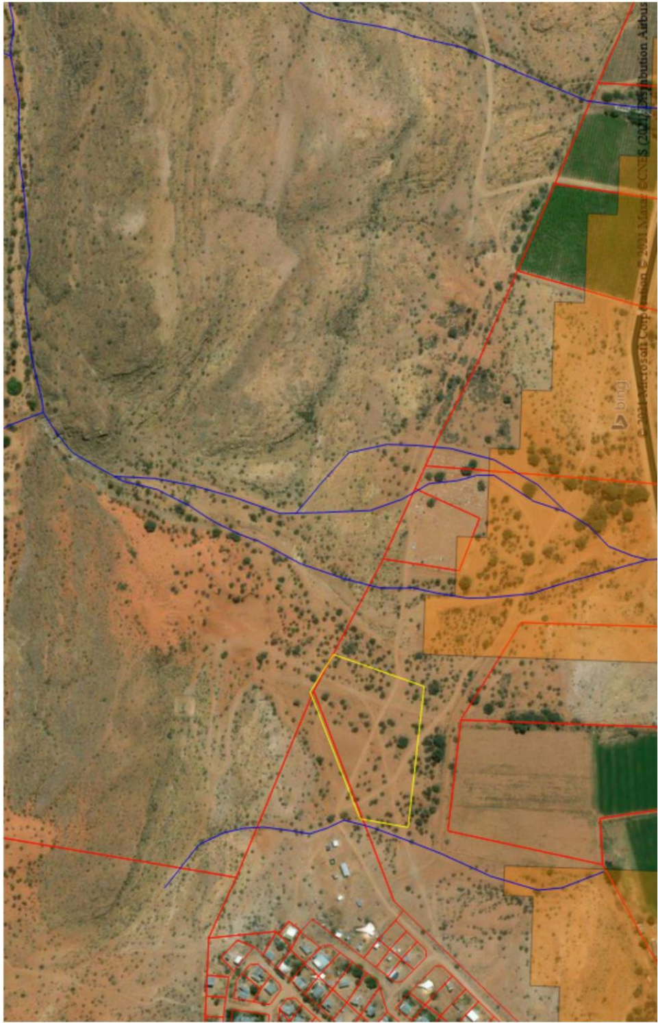
Map 1: Locality map of the proposed construction of a graveyard in Lutzburg, Northern Cape Province. Note that the site does not fall within the Lower Gariep Alluvial vegetation type, a Threatened Ecosystem. Note also extensive transformation of the surroundings due to agriculture. The small drainage line bordering the site to the west and larger drainage line to the east are also indicated. The urban area of Lutzburg is visible to the west of the site.
