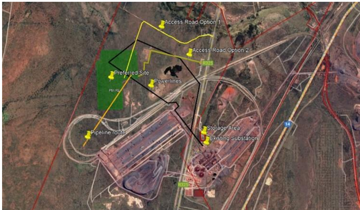
Figure 14: Overall Layout of the PV Solar Plant
