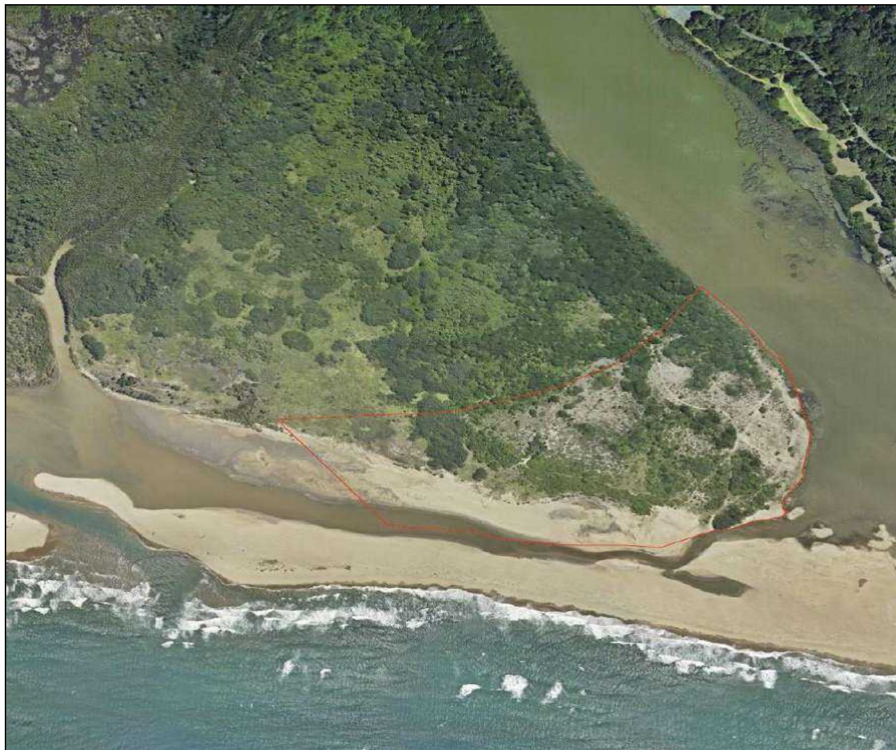
Figure 8b Project area of dredge spoil where GEF funding was received to remove 1.5 million m 3 to restore and improve connectivity between the uMfolozi river and the Lake St Lucia
