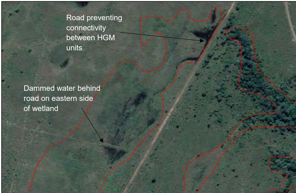
Figure 1.10 - 2017 Google Earth satellite imagery showing disruptions to hydrological flows in wetland and the preferential flow on the eastern side of the HGM unit during wet season.
