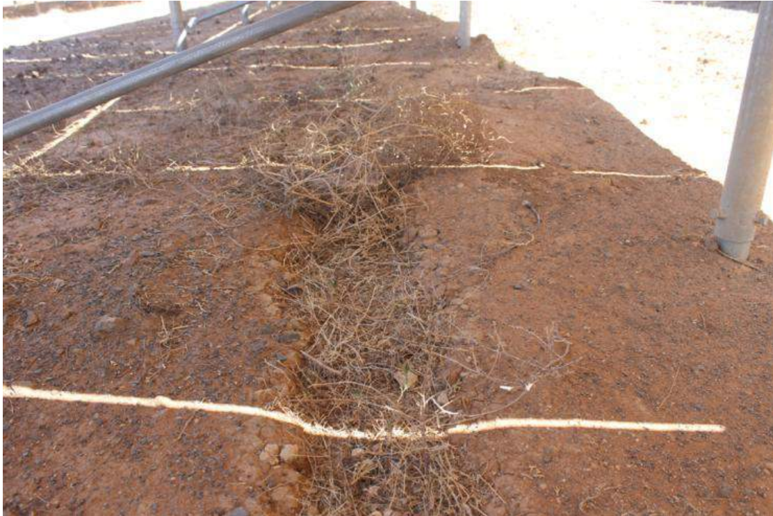
Figure 23. Image indicating rilling and plant invasion in rill under PV module. Habitat form and structure will change on site as a consequence of the establishment of PV modules
