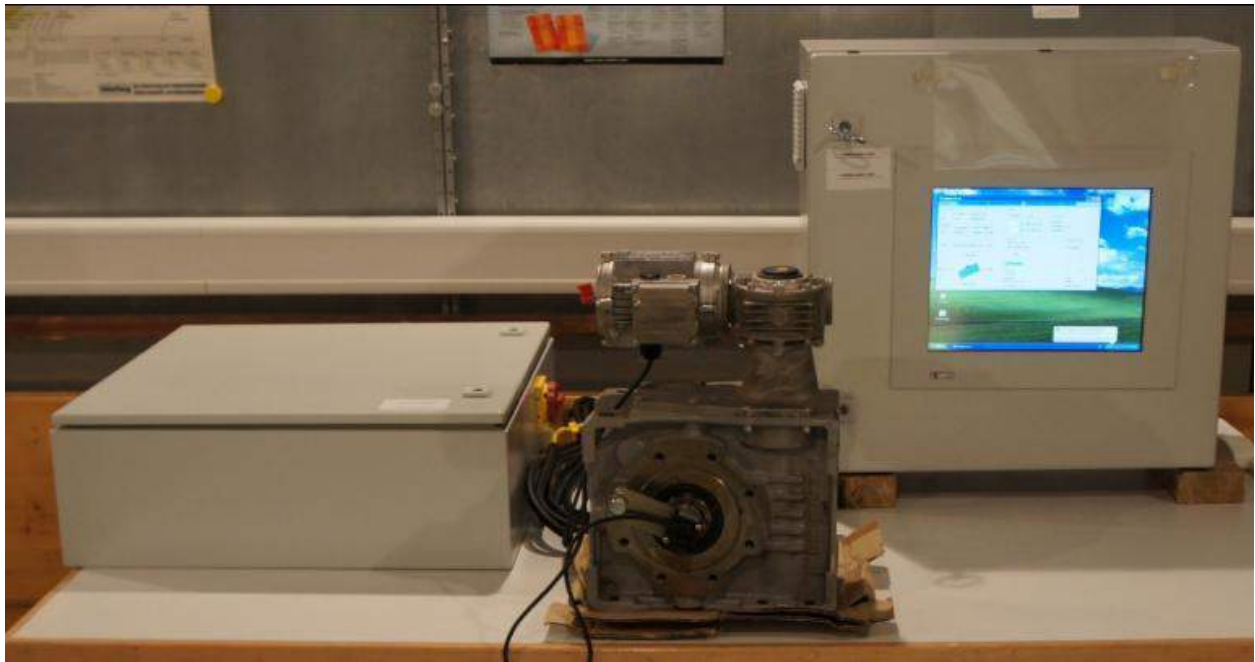
Figure 2: Tracker and DC combiner test set-up
