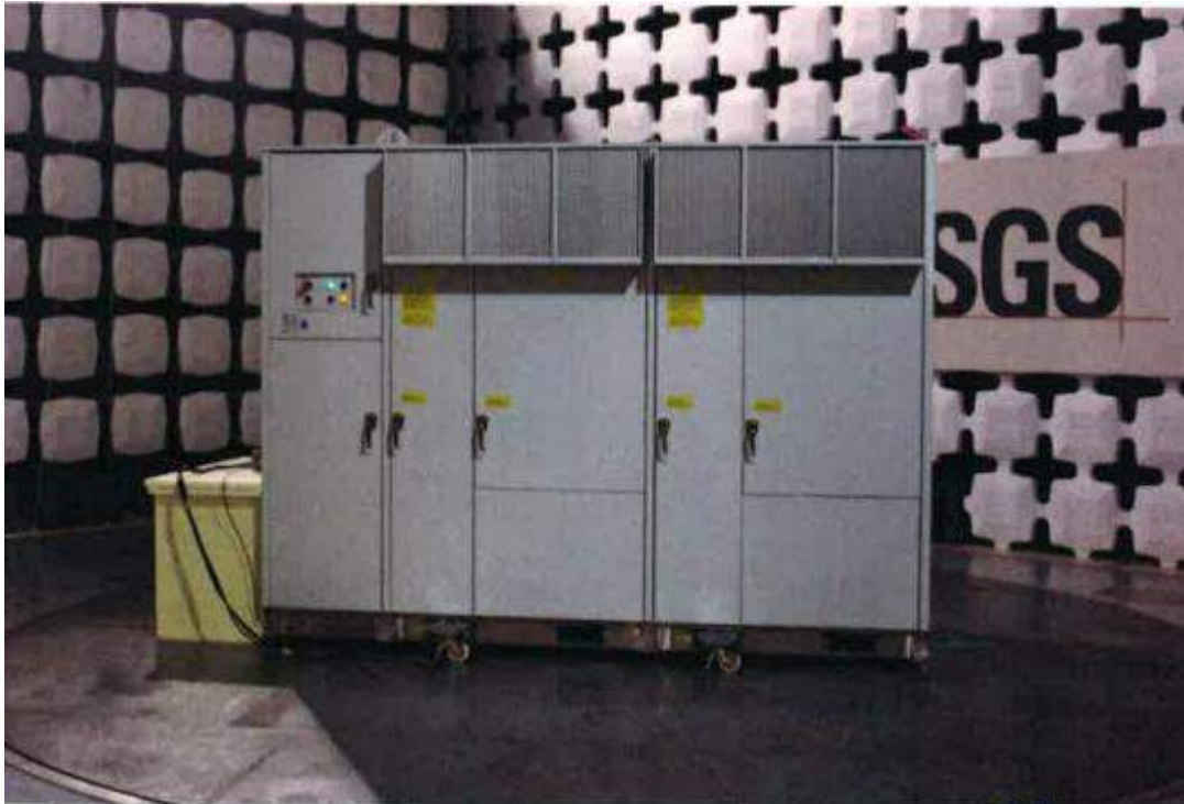
Figure 4: Inverter test set-up
