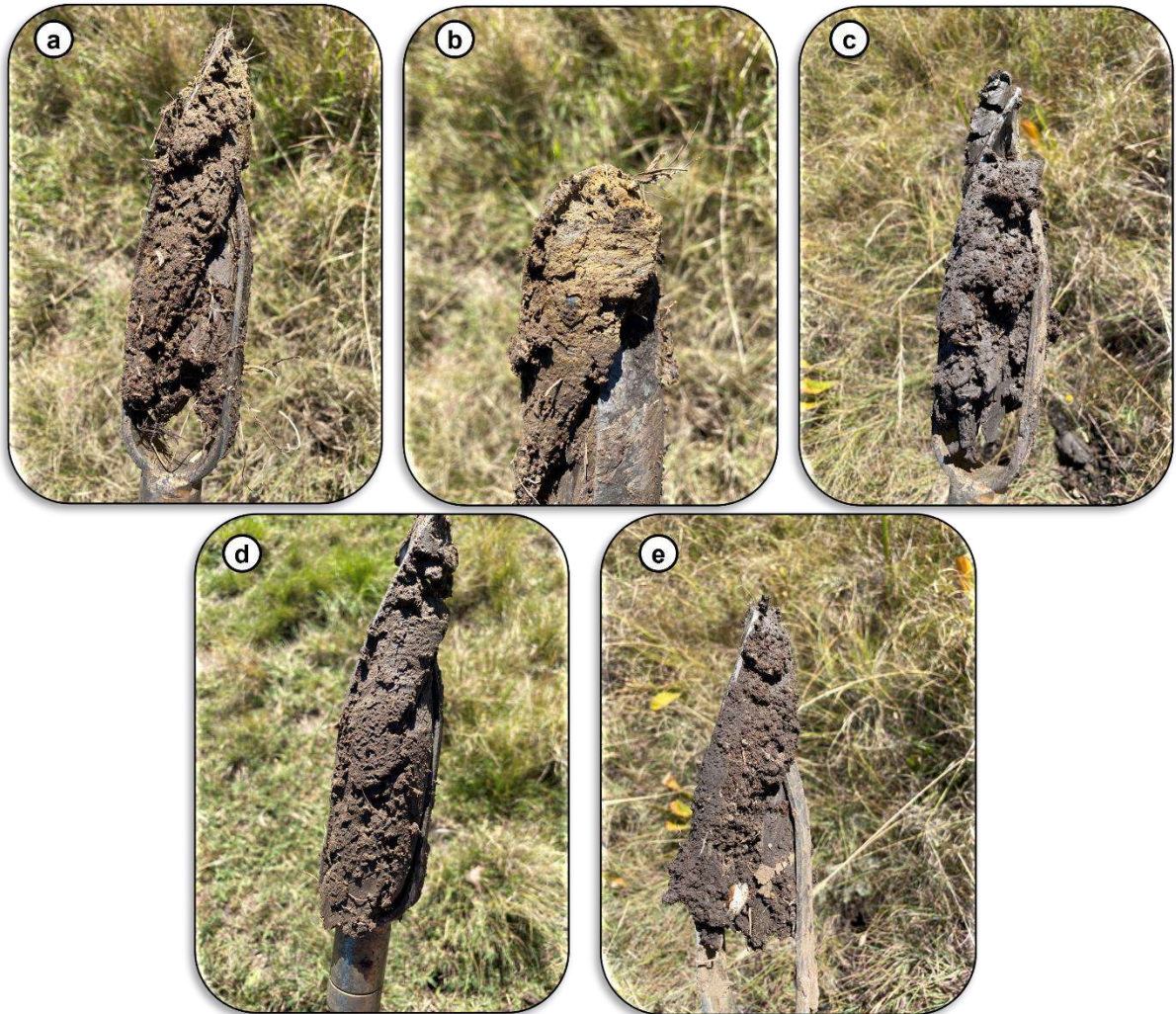
Figure 29: Typical soils associated with the proposed Oslaagte Solar 1 PV. Photographs (a) and (b) indicating the Sepane soils, photograph (c) indicating the gleyed content within the Valsrivier soils. Additionally, photographs (d) and € indicating the Bonheim soils
