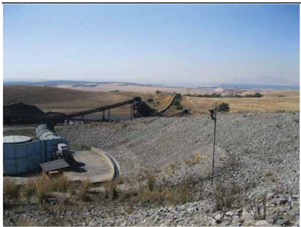
Figure 2.9 Typical Conveyor Belt System in the Background Transporting Coal to a Wash Plant
