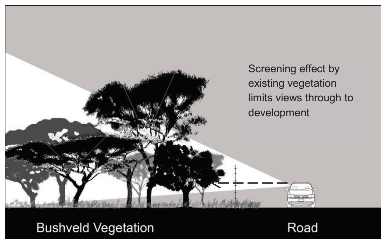
Figure 6-21: Section illustrating the screening effect of vegetation which increases the Visual Absorption Capacity of the Landscape
