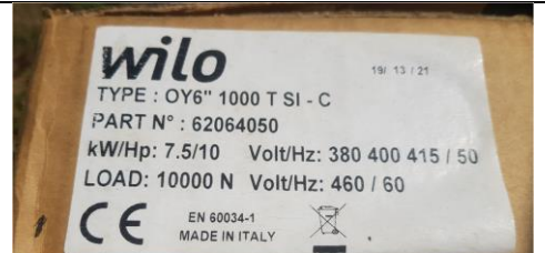
Thorndale dam pump information
