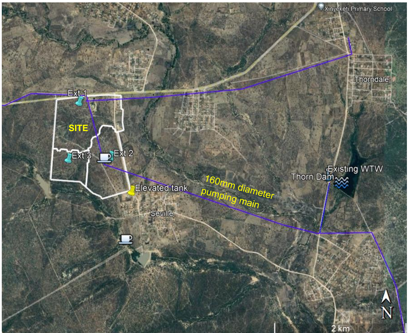
Figure 11 Water bulk lines
